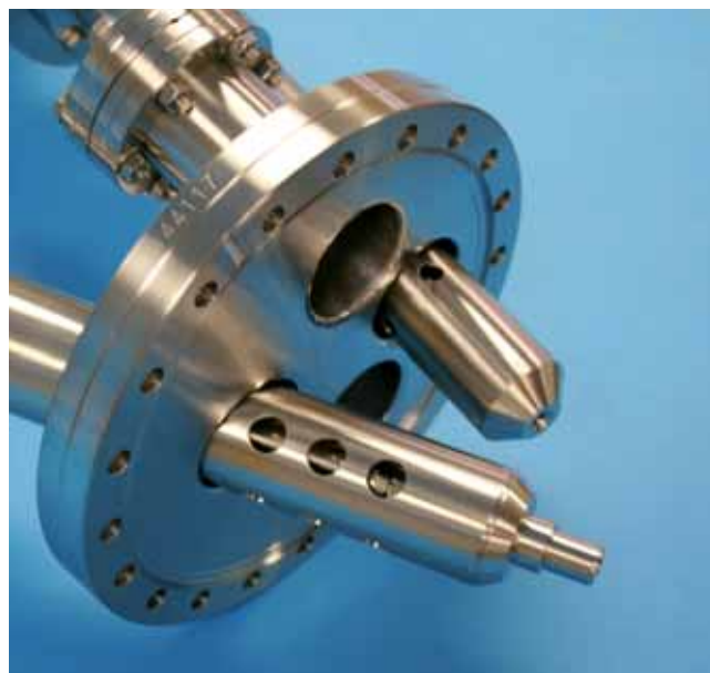
A complete SIMS facility mounted on a single conflat flange
