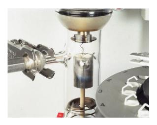
Custom designed hot-zone inlet for the PerkinElmer Pyris TGA system. Includes optimised 'hot-zone' sampling connection.
