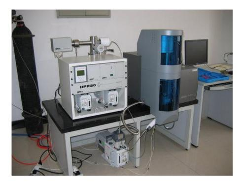
Custom designed hot-zone inlet for Setaram TGA system. Includes optimised 'hot-zone' sampling connection and heated filter assembly and support.
