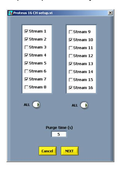
Multi stream sampling enables a single mass spectrometer to analyse sample from up to 80 streams in a continuous loop sequence.
