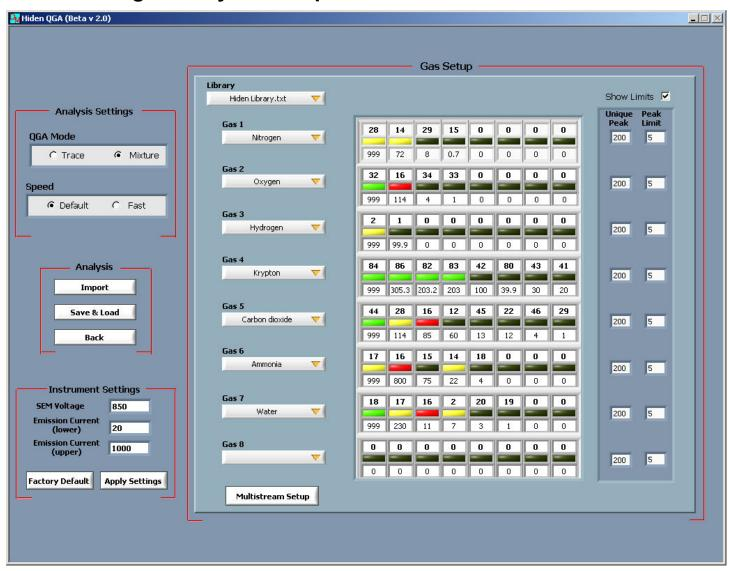
Each template file is set up using the mass spectral library calculator.
