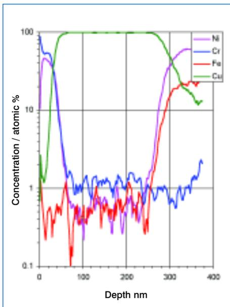
The example shows a quantified depth profile through a NiCr/Cu/NiFe layer structure. The primary ions were 5 keV Ar<sup>+</sup> from the Hiden IG20 gas ion gun.
