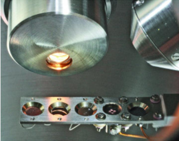
The Hiden MAXIM quadrupole SIMS analyser is a state of the art secondary ion mass spectrometer for static and dynamic SIMS applications.
