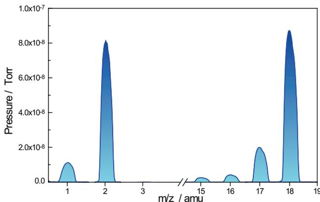
Low mass performance of the 3F system 6mm pole diameter - 50 amu mass range system. Excellent abundance sensitivity and peak separation over the entire 1- 50 amu mass range.
