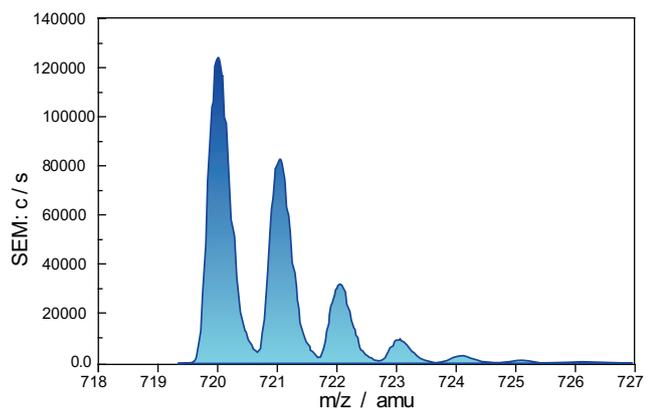
High mass performance of the 3F system, 9mm pole diameter - 1000 amu mass range system. C60 peak at mass 760 with natural abundance carbon isotope peaks at mass 721, 722, 723 and 724....
