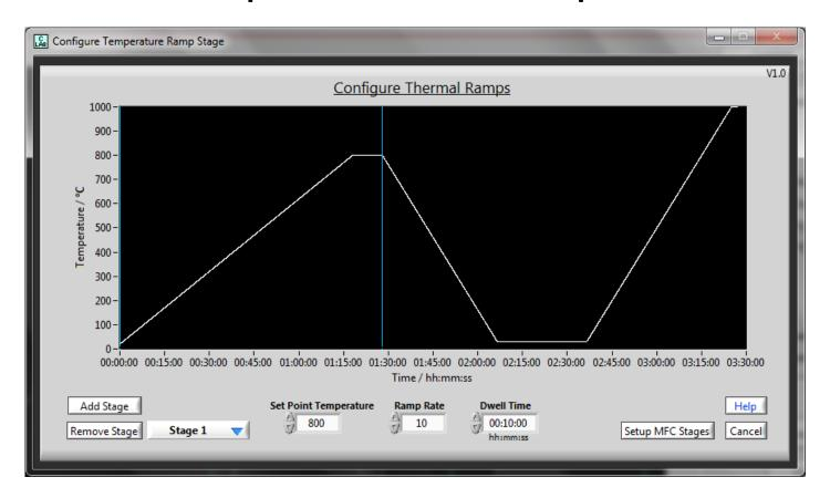
Stage 1: Configure the temperature profile of the experiment
