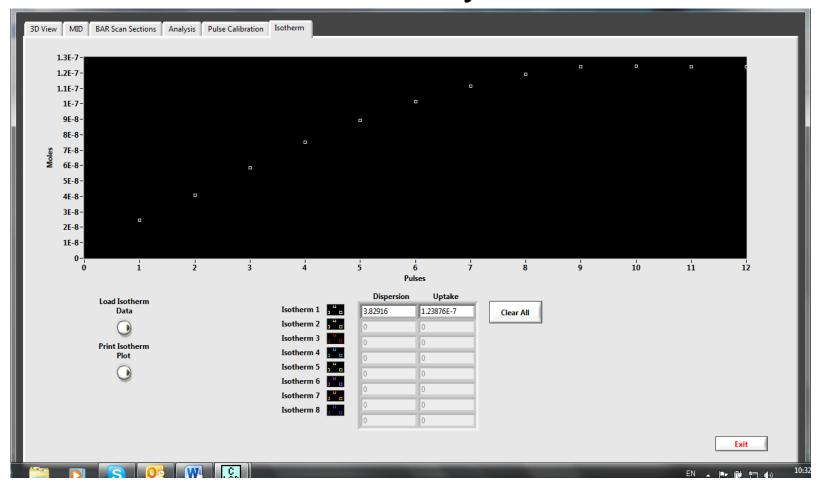
Calculate and plot the pulse adsorption isotherm.
