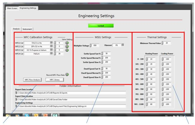
Control and calibration of MFCs for different gases
