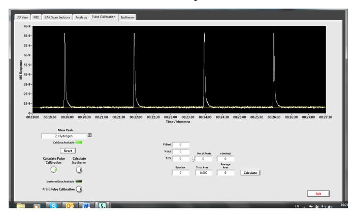
Calibrate MS response vs injected gas amount for quantification of desorbed gases.
