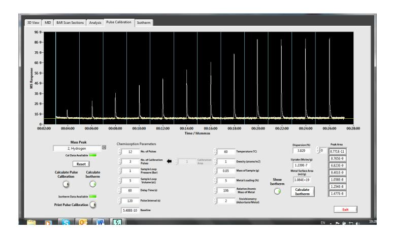
Pulse chemisorption algorithms to determine total uptake, metal surface area and dispersion from pulse adsorption experiments.
