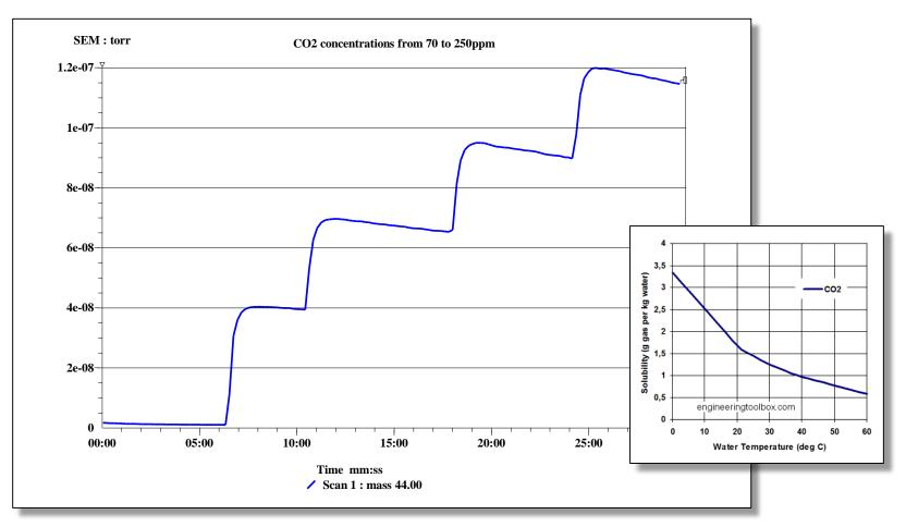
The figure shows the addition of 10mL aliquots of a  $CO_2$ -satured  $H_2O$  solution (1.5g  $CO_2$  per 1 kg  $H_2O$  at 23 deg C as per inset graph) to 200 mL pure  $H_2O$ . Therefore, the concentrations of  $CO_2$  are approximately 0, 70,140, 200, and 250 ppm for the 5 time steps shown.
