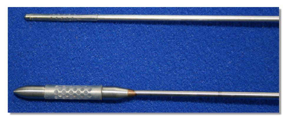
A comparison of the two Dissolved Species Probes. The larger tip is specifically designed for looking at gaseous species in soils, sands and semi-solid moist environments. Both probes are 0.5m in length.
