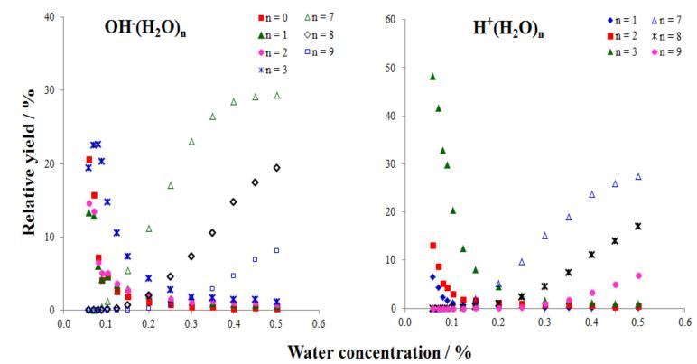
Water concentration has a marked effect on the appearance of both positive and negative ion clusters. With higher water concentration producing larger ion clusters.
