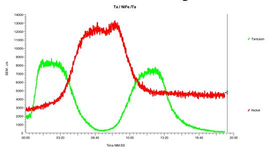
The IMP EPD data shows the depth resolution achieved in an ion mill of a:
