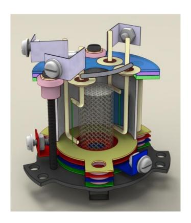
Source cage +3volts (Range 0 to 10volts)
