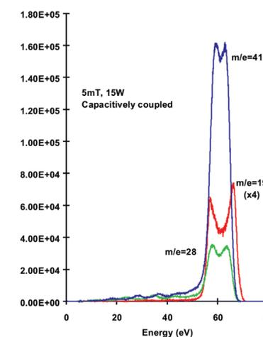
Typical IEDs are shown in the figures. The spectra show the energy distributions for mass resolved ions as indicated. The energy range of the instrument is 100 eV with an option for 1000 eV operation. The energy spectrum can be used to determine the plasma potential, tailing on the energy spectra is an indication of collisions taking place in the plasma sheath.
