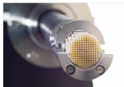
Intra-catalyst sampling of gas and temperature
