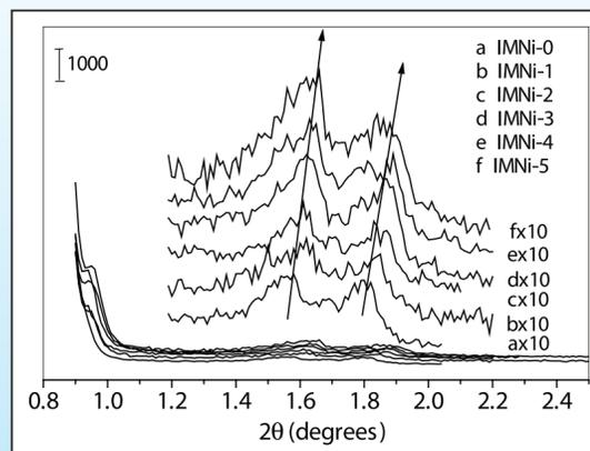
Figure 5: Low-angle XRD patterns of nickel-containing mesoporous silicas after each impregnation cycle
