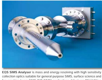
EQS SIMS Analyser is mass and energy resolving with high sensitivity collection optics suitable for general purpose SIMS, surface science and focussed ion beam SIMS (FIB-SIMS) applications. It features DN63 fitting with on-axis collection and a 45° electrostatic sector energy filter. Customised lengths are available.
