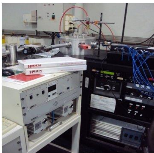
Figure 1. HPR-30 Vacuum Process Gas Analyser coupled to RIE plasma etch.
