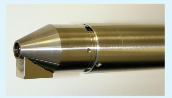
The filament is housed in the box structure on the underside of the probe and has no line of site to the sample. The electrons, with energy variable between 4 and 150 eV, are directed into the ionization cage visible at the end of the device.
