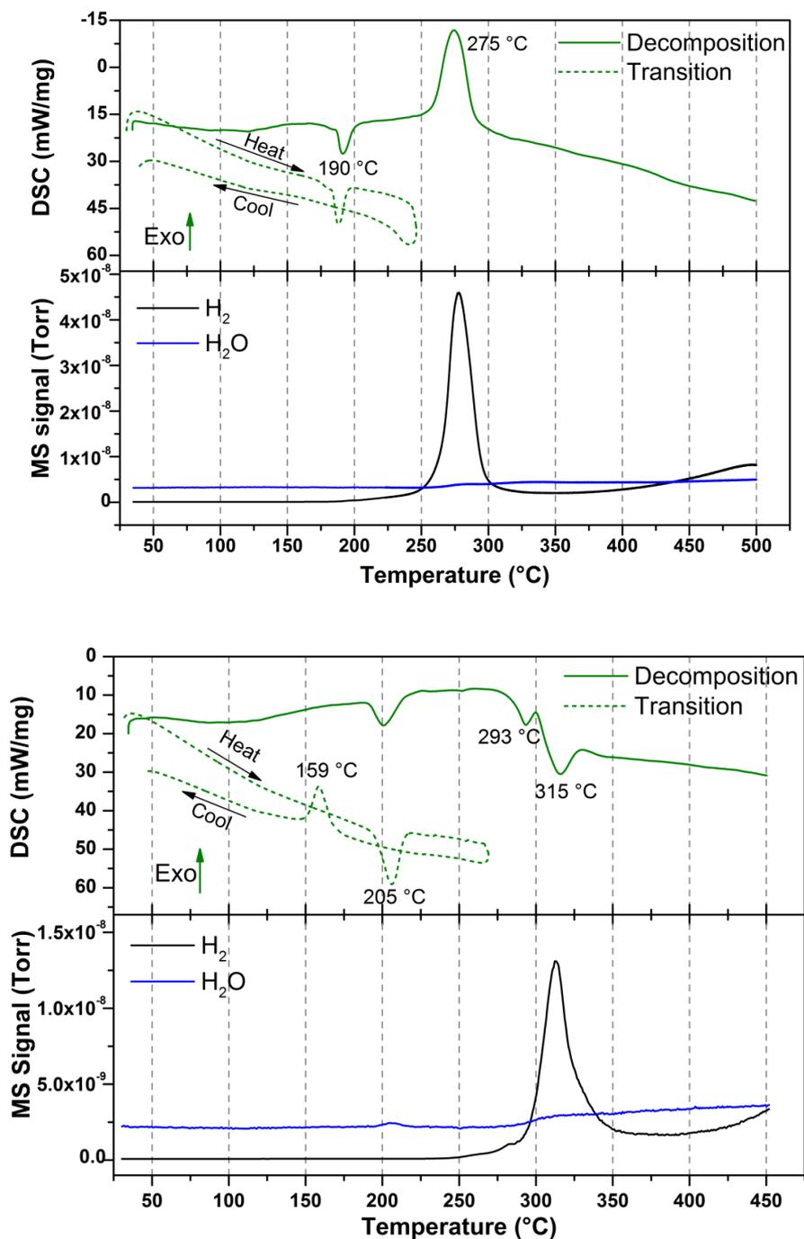
Differential scanning calorimetry (DSC) and mass spectroscopy (MS) data of Ag<sub>2</sub>B<sub>10</sub>H<sub>10</sub> (**top**) and Ag<sub>2</sub>B<sub>12</sub>H<sub>12</sub> (**bottom**). Two DSC measurements are shown for each material, one illustrating decomposition (solid line) and another showing the polymorphic phase transformation (dashed line). The MS trace is shown in the bottom part of the graphs.
