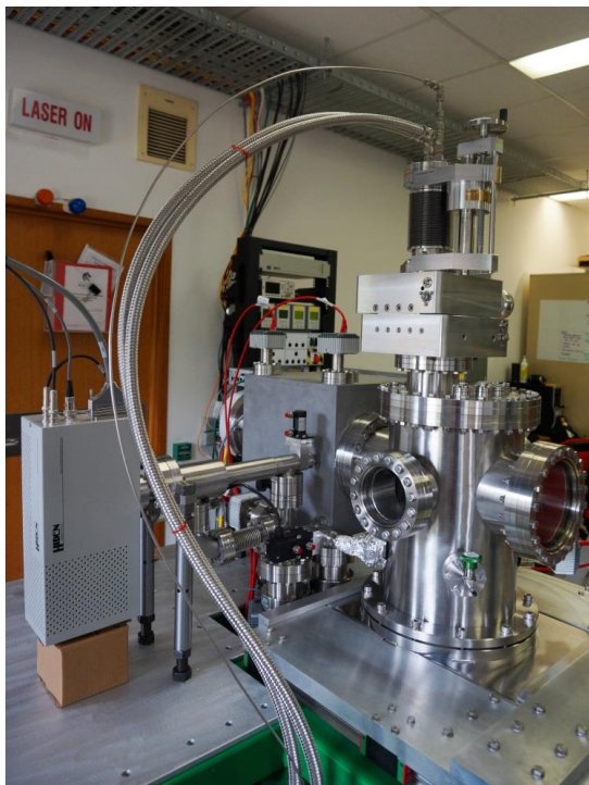
Figure 1. The Mk II scanning helium microscope (SHeM)
