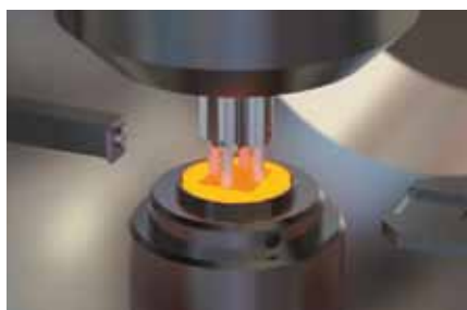
TPD Workstation with hot sample
