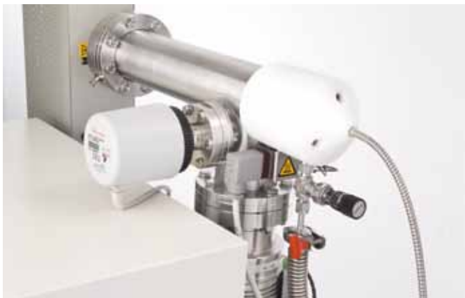
HPR-20 QIC TMS transient MS QIC inlet
