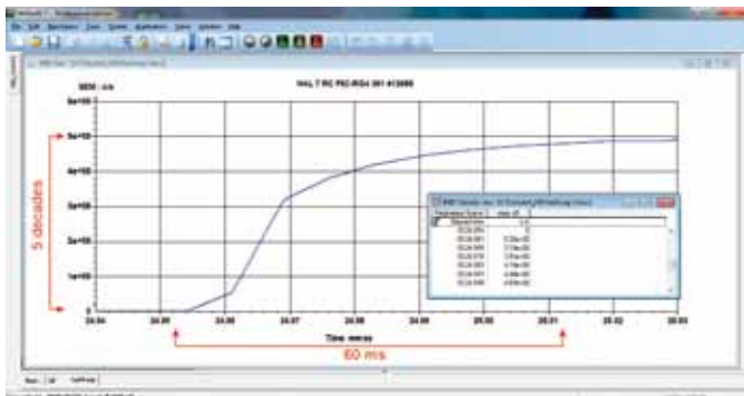
HPR-20 transient MS data - > 5 decades response in < 100 ms
