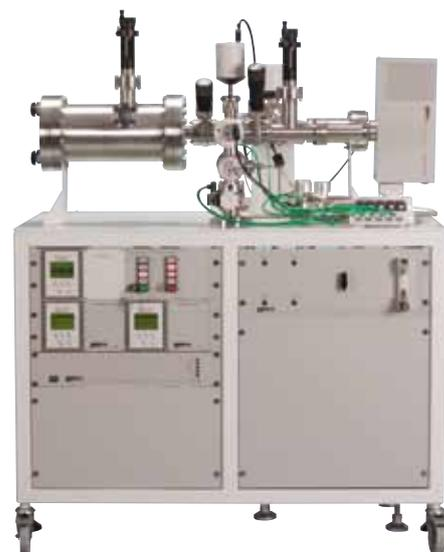
**HPR-90** automated package cracking analysis system
