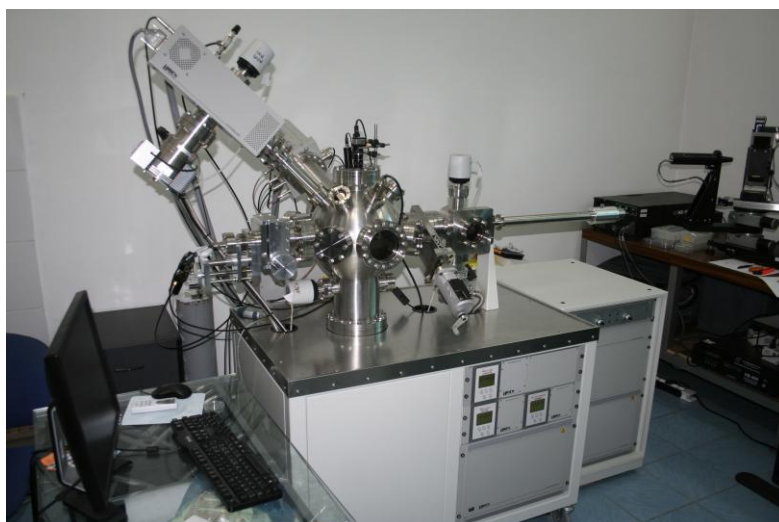
The Hidden MAXIM SIMS/SNMS Workstation in the National Institute for Lasers, Plasma and Radiation Physics, Bucharest Romania
