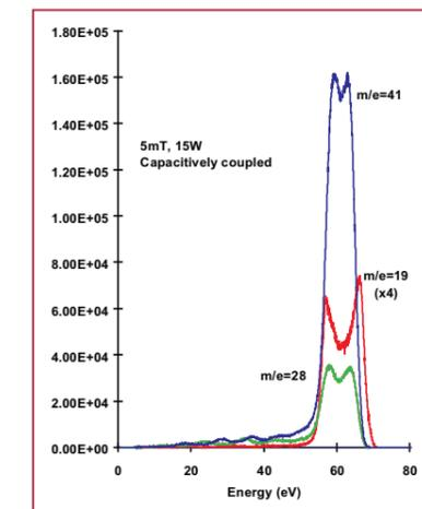
Typical IEDs are shown in the figures. The spectra show the energy distributions for mass resolved ions as indicated. The energy range of the instrument is 100 eV with an option for 1000 eV operation. The energy spectrum can be used to determine the plasma potential, tailing on the energy spectra is an indication of collisions taking place in the plasma sheath.
