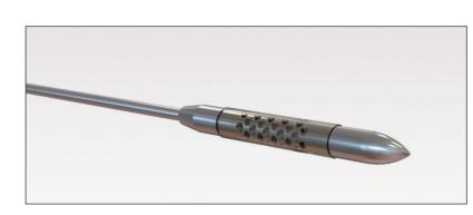
Direct membrane inlet probe – 500 mm long, for analysis of dissolved species in fermentation cultures, soil samples, and general applications where analysis of dissolved species in a liquid sample is required.
