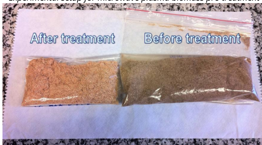
Sugar cane bagasse, raw material (right) and after 6 hours of treatment (left)
