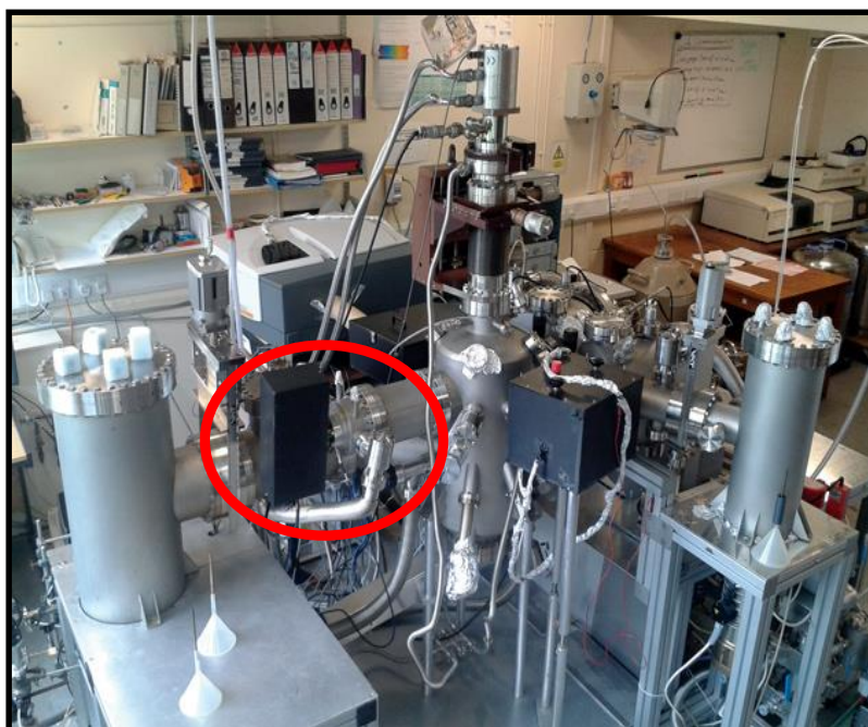
Figure 1: The Heriot-Watt University laboratory astrochemistry experimental ultrahigh vacuum chamber with the Hidden QMS outlined in red.
