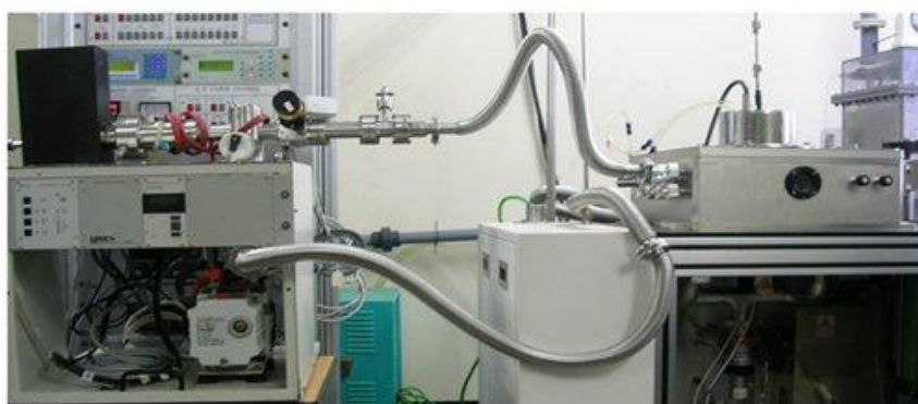
Fig. 1 Photograph of the Hidden Mass Spectrometer in use in our lab
