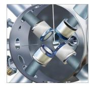
The experimental setup with four essentially balanced planar magnetrons (2" Ti targets), Langmuir probe, and the system of capillaries used to introduce wires from atmospheric pressure.
