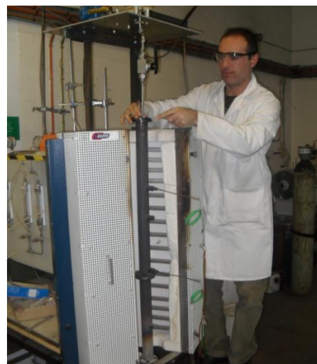
Figure 2 Fluidised Bed Reactor used for the spent grains pyrolysis.
