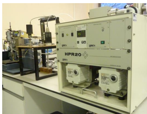
Figure 1: Flow adsorption calorimetry instrumentation. The flow-through Setaram DSC111 differential calorimeter is visible on the extreme left. The sample tube is held vertically in the stainless steel furnace. The automated gas sampling valve is held on the platform. The low-flow capillary interface to the Hidden HPR-20 Mass Spectrometer can be seen under the valve platform. The tube furnace alongside the calorimeter is for catalyst activation.
