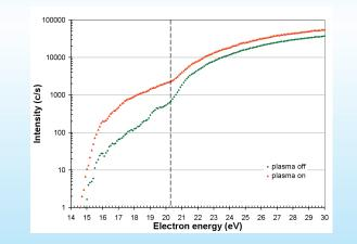
Fig 7. Appearance potential scans for O with the plasma on and off. The threshold for the dissociative ionisation of  $O_2$  is 20.3eV.
