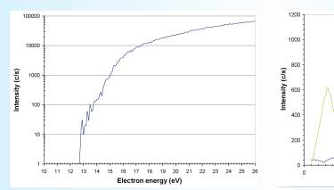
*Fig 9. Appearance potential of*  $O_3^+$ produced in a commercial ozone generator.
