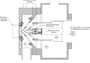
*Fig 2. Schematic of the Hiden* Modulated Beam Mass Spectrometer System. The three cones are fitted with apertures of 0.2mm at the first stage, 0.3mm at the second stage and 1.0mm at the entrance of the EQP mass/energy analyser.
