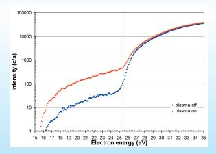
Fig. 8. Appearance potential scans for N with the plasma on and off. The threshold for the dissociative ionisation from  $N_2$  is 25.2eV.
