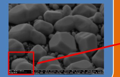
Vibrational effects of the additional pumping system with the Hiden SIMS probe is seen in the SEM image of the gold cluster on carbon sample at 200kX magnification.
