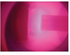
for ion detection. This detector provides high sensitivity, fast response and high dynamic range (> $10^{10}$ ) for plasma ions and neutrals. Mass range options are 300 amu, 510 amu,1000 amu and 2500 amu. An energy range of 100 eV is standard and 1000 eV optional to provide the user with analysis of positive and negative ions and appearance potential spectra for radicals analysis. Signal gating by direct TTL input is also available with gating resolution to 1  $\mu s$  for afterglow studies.
