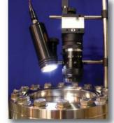
Normal incidence lighting and camera for undistorted view.
