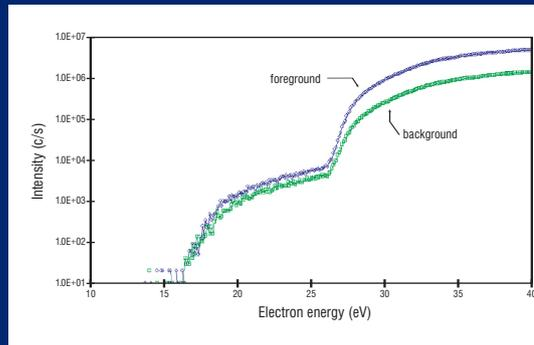
Threshold Ionisation curves of  $N^+$  obtained from an atmospheric pressure helium discharge operating in ambient air.
