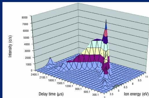
Time resolved Ion Energy Distribution generated automatically by software controlled scanning of the timing parameters (delay and gate) from within MASsoft.
