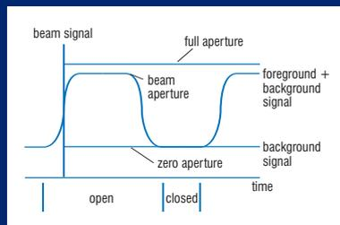
The resultant 'beam only' signal, which is directly proportional to radical number density, is identified automatically, providing rapid and accurate quantification of key species.
