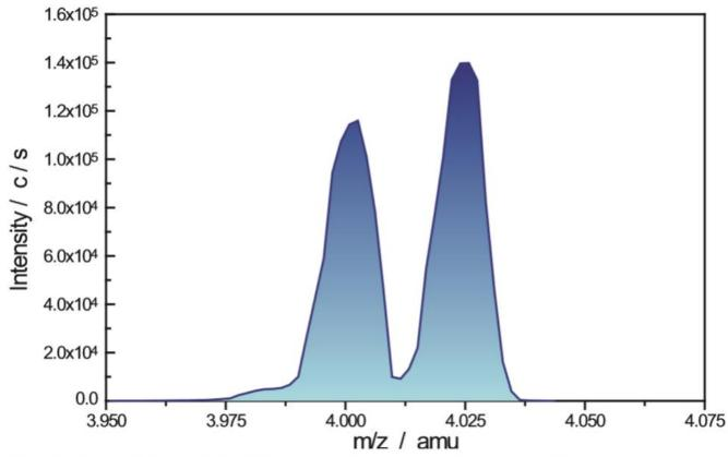
Ultra high resolution of the 3F system, 9mm pole diameter - 50 amu mass range system. Separation of the helium and deuterium peaks with a difference of only 0.0256.
