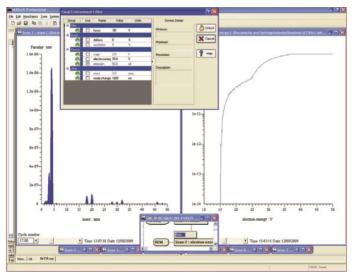
DLS-1, real time TIMS data taken at JET, UK. Spectra shows scans at 3amu, separating <sup>3</sup>He from <sup>1</sup>H<sup>2</sup>D. Mass separation: 0.0058 amu
