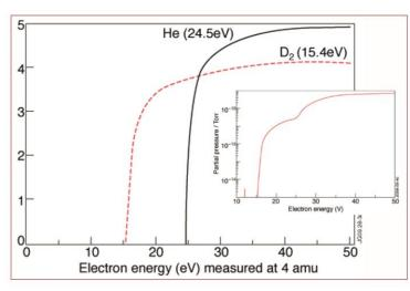
DLS-1, real time TIMS data taken at JET, UK. <sup>2</sup>D<sub>2</sub> and <sup>4</sup>He are easily separated and quantifiable
