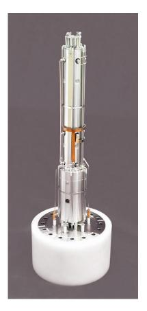
Quadrupole Mass Spectrometers for Advanced Science
