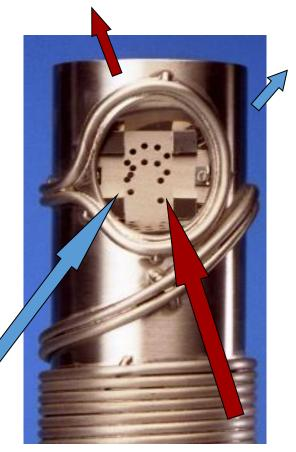
XBS Probe Tip + Beam Apertures
