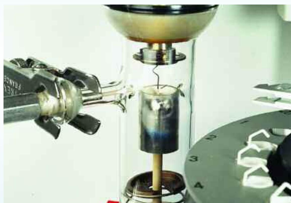
Fig 3a. TGA Interface for PE Pyris TGA Custom designed Hot zone inlet for the PerkinElmer Pyris TGA system. Includes optimised 'Hot-zone' sampling connection
