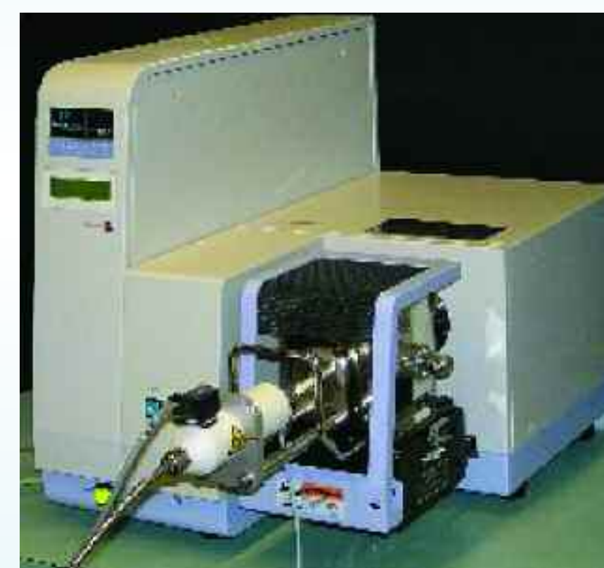
Fig 3b. TGA Interface for PE Diamond TGA Custom designed Hot zone inlet for the PerkinElmer Diamond TGA system. Includes optimised 'Hot-zone' sampling connection and heated filter assembly.
