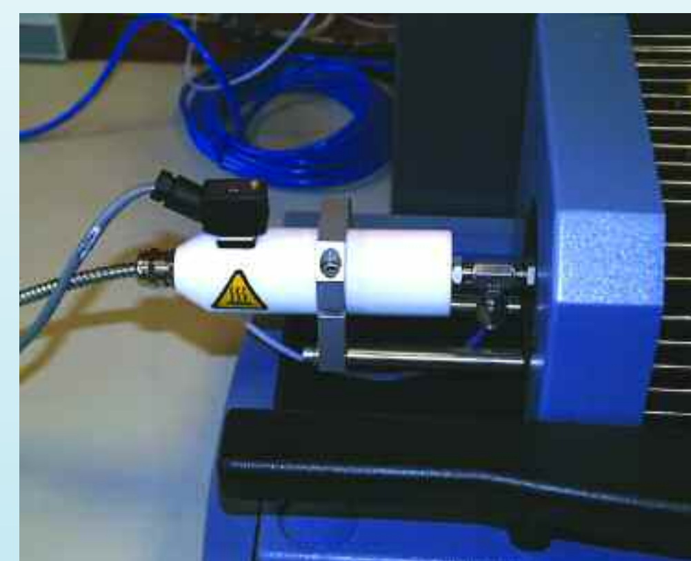
Fig 4b. TGA Interface for TA Instruments Q600 Custom designed Hot zone inlet for the TA Instruments Q500 TGA system. Includes optimised 'Hot-zone' sampling connection and heated filter assembly and support.
