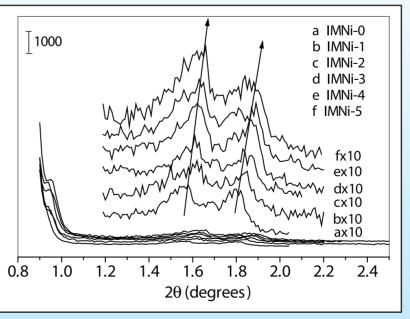
Figure 5: Low-angle XRD patterns of nickelcontaining mesoporous silicas after each impregnation cycle (a) 0 cycles, (b) 1 cycle, (c) 2 cycles, (d) 3 cycles, (e) 4 cycles, (f) 5 cycles.
