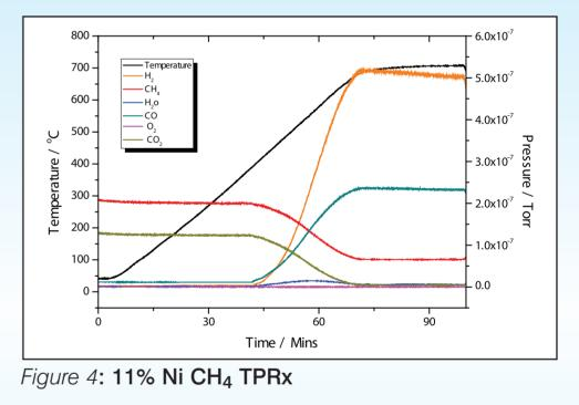
In the 11 % Ni sample, conversion of  $CH_4 + CO_2 \rightarrow 2H_2 + 2CO$  occurs at around 400°C with complete conversion of the CO<sub>2</sub> occurring at a similar temperature of the 5% sample at around 700°C
