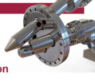
The Hiden Modular SIMS is used in MBF for surface analysis, offering crucial data on material composition, structure, and growth.
