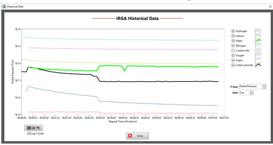
A trend analysis view showing the partial pressure of all gases as a function of time is available during live data acquisition and for viewing previous runs as a historical data view.
