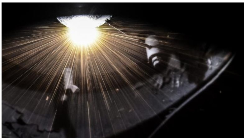
Figure 2. Visual observation of the arc spot on the Mo 0.79 Cu 0.21 cathode
