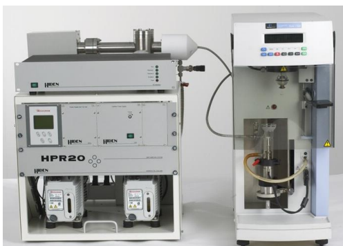
Pyris 1 TGA interfaced to the HPR20 QIC
