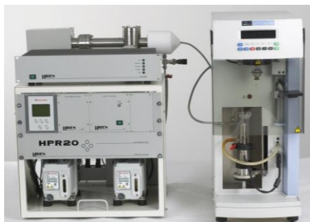
HPR-20 interfaced to the STA6000
