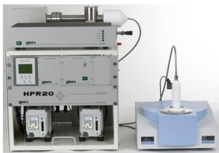
HPR-20 interfaced to the Pyris 1 TGA
