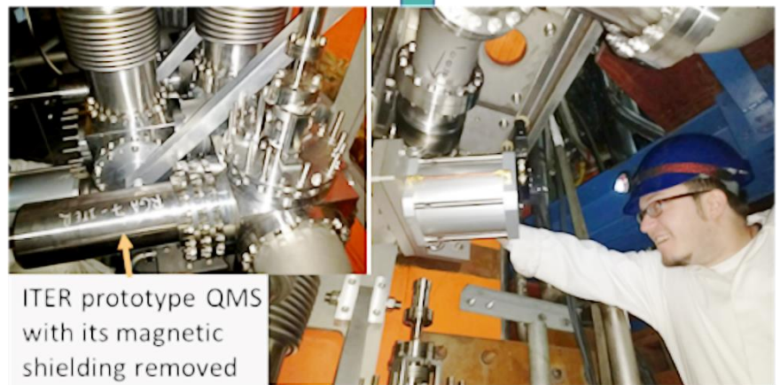
Figure 1. Paper co-author Ionut Jepu (right photo) pointing to location of the ITER-compatible Hiden QMS unit (left photo) which is part of the multi-sensor, neutral gas analysis station located under JET's fusion plasma containment torus, to sample the gas composition on the sub-divertor region (top image). Credit: EUROfusion Consortium.
