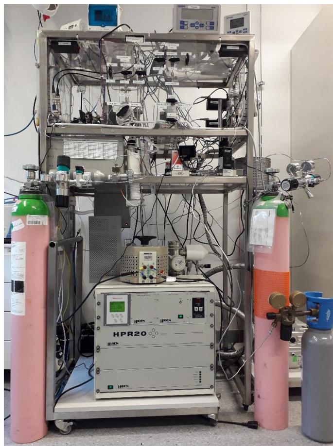
*Experimental setup for catalytic tests equipped with Hidden HPR-20 QMS detector.*
