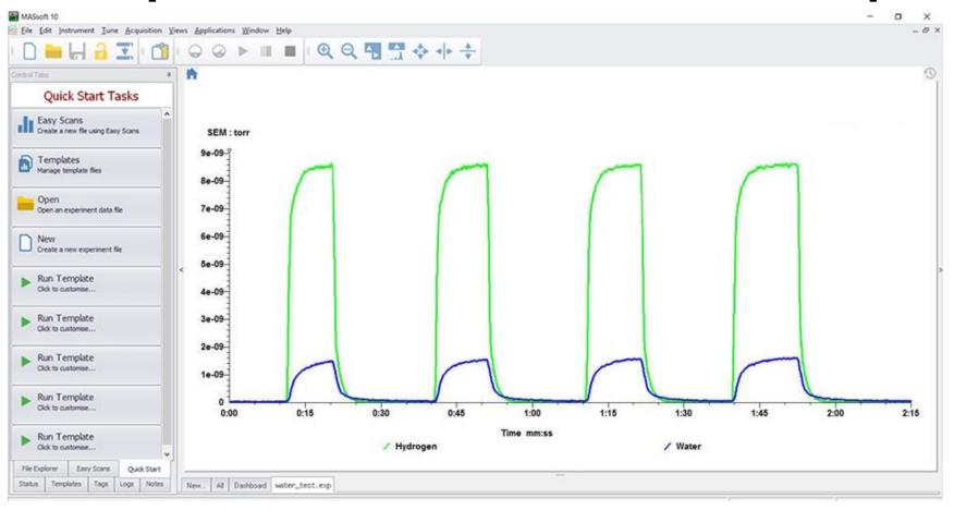
Data shows the response of the QIC inlet to gas and vapour during switching between a dry He stream and a wet  $H_2$  and Ar flow. For clarity, only the  $H_2$  and  $H_2$ O data is shown in the graph.
