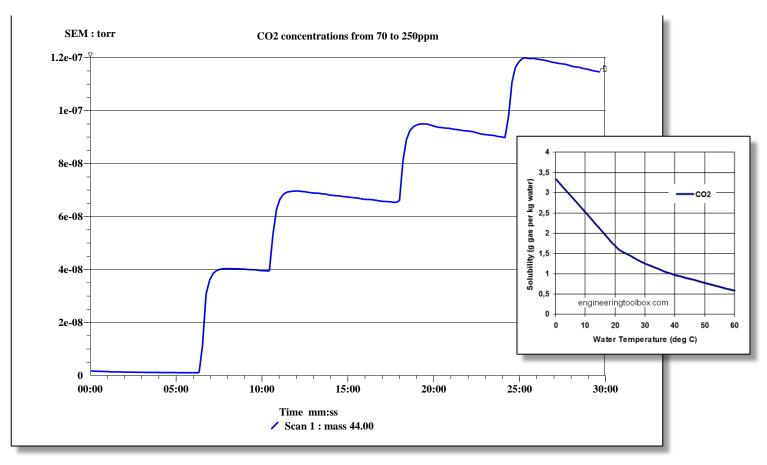
The figure shows the addition of 10mL aliquots of a  $CO_2$ -satured  $H_2O$  solution (1.5g  $CO_2$  per 1 kg  $H_2O$  at 23 °C as per inset graph) to 200 mL pure  $H_2O$ . Therefore, the concentrations of  $CO_2$  are approximately 0, 70 ,140, 200, and 250 ppm for the 5 time steps shown.
