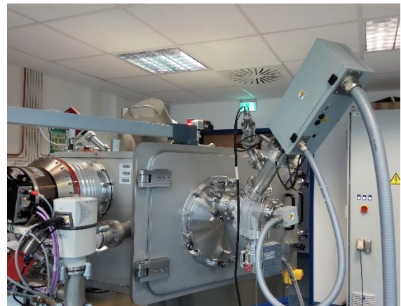
Figure 1: Typical configuration of an experimental setup with energy-selective mass spectrometer (EQP 300) at the Leibniz Institute for Surface Engineering. The setup was used for the characterization of a commercially available Kaufman-type ion beam source.
