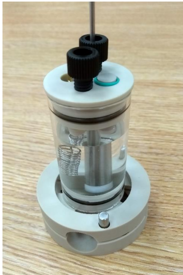
Figure 8: DEMS probe fitted inside Redox.me cell
