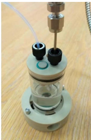
Figure 9: Ultra Low Flow capillary connected to Redox.me cell
