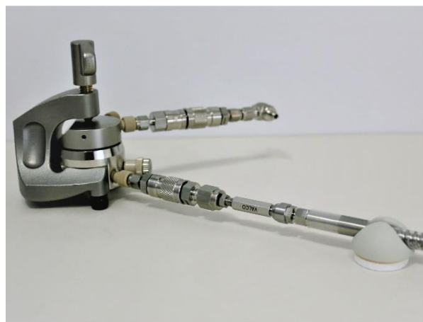
Figure 10: ULF connection to ECC-DEMS cell, with quick connects
