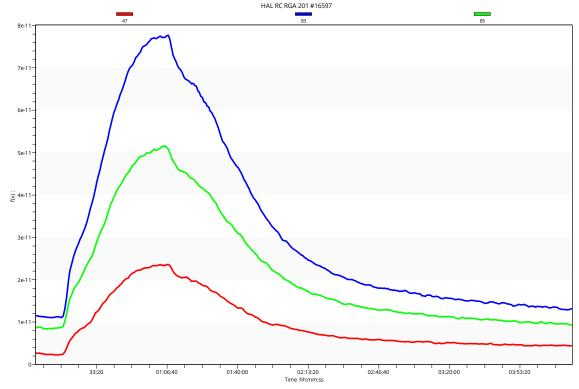
Response of 1.29ppb chloroform, measured at mass 83, was 6.6e-11. Noise in this range is 1e-13, suggesting detection limits of approximately **20ppt**.
