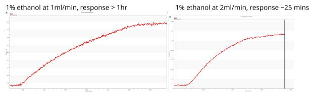
Results suggest that there is a significant increase in response time at flow rates lower than 2 ml/min. Response time decreases as flow rate increases. There is no effect from flowrate on sensitivity.
